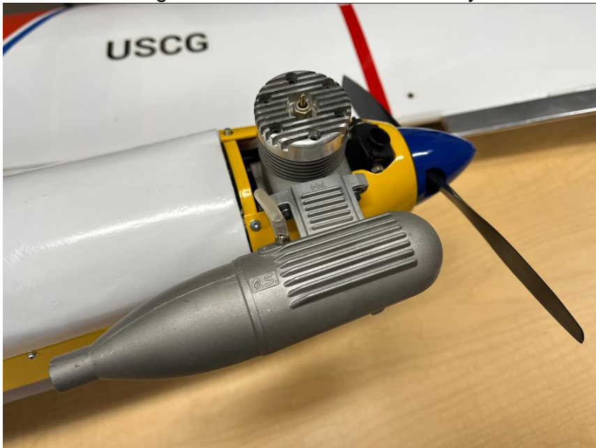
An excellent engine. Note the aftermarket Perry carburetor.
