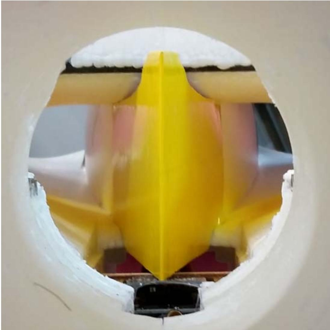
View up the tailpipe with the fan removed showing the “wedge of cheddar” mod to the inlet ducting.
